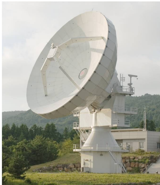
FIG. 1.—Photograph of the 21 m diameter KVN Tamna radio telescope. See the electronic edition of the PASP for a color version of this figure.
