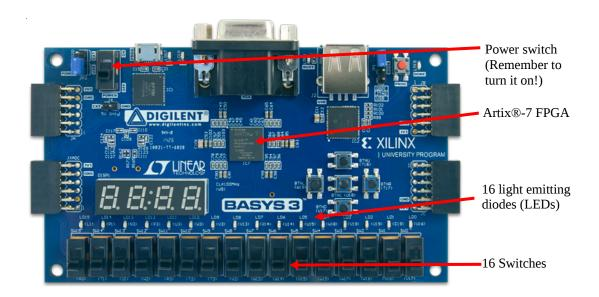
This board includes, among other devices, a Artix®-7 FPGA chip which we can program, some switches, some light-emitting diodes (LEDs), and some other cool features. You can learn more about the Basys 3 Starter Board from:
